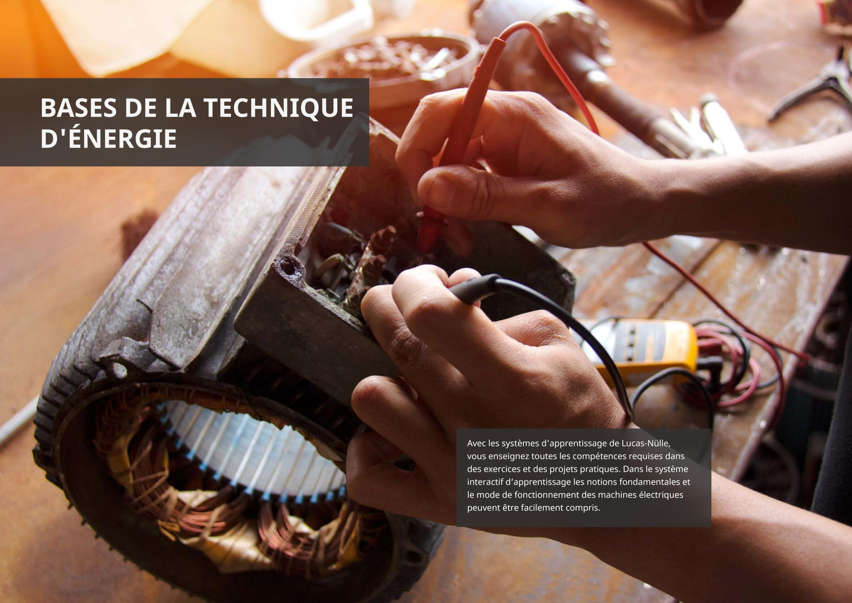
A close-up photograph of a person's hands using a multimeter to test an electric motor. The multimeter is yellow and black, and the person is holding its red and black probes. The motor is partially disassembled, showing its internal stator windings and rotor. The background is a workshop with various tools and equipment.
