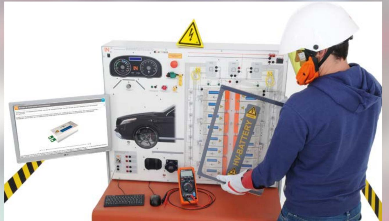
Opening a HV battery for repair
