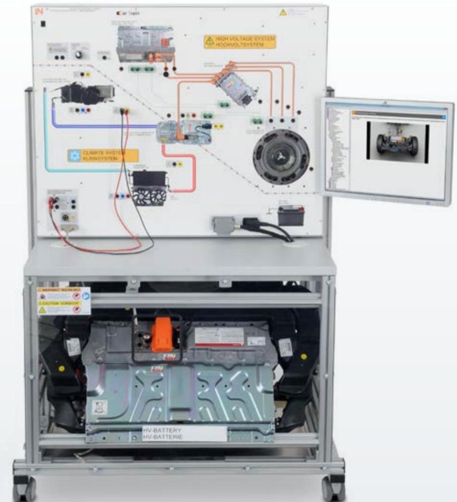
Combined equipment for the topics of hybrid drive trains and high voltage air conditioning in vehicles. Trainees can use the set to learn about the aspects of servicing, diagnostics and repair of high-voltage networks and air conditioning.
