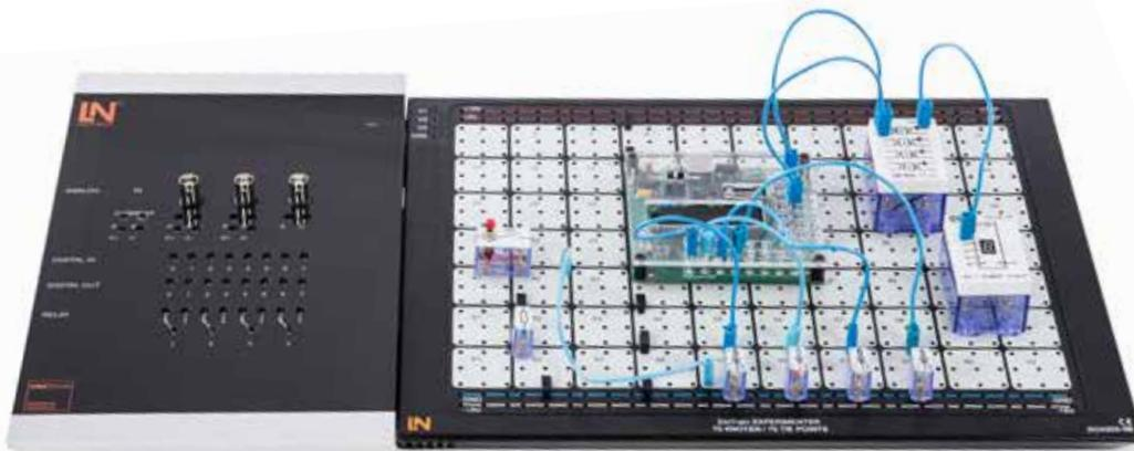
Interface with EloTrain experimenter for plug-in modules
