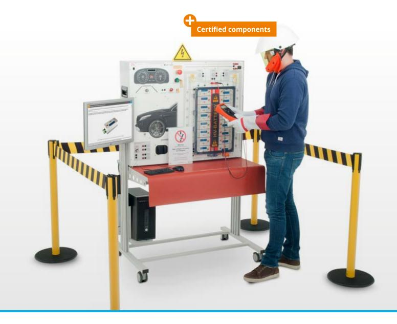
Students work directly on a high-voltage battery. The system is setup to work exactly like a real working high voltage battery. Students can take measurements and troubleshoot all the way down to the actual cells that even includes how to replace and repair a high-voltage battery.
