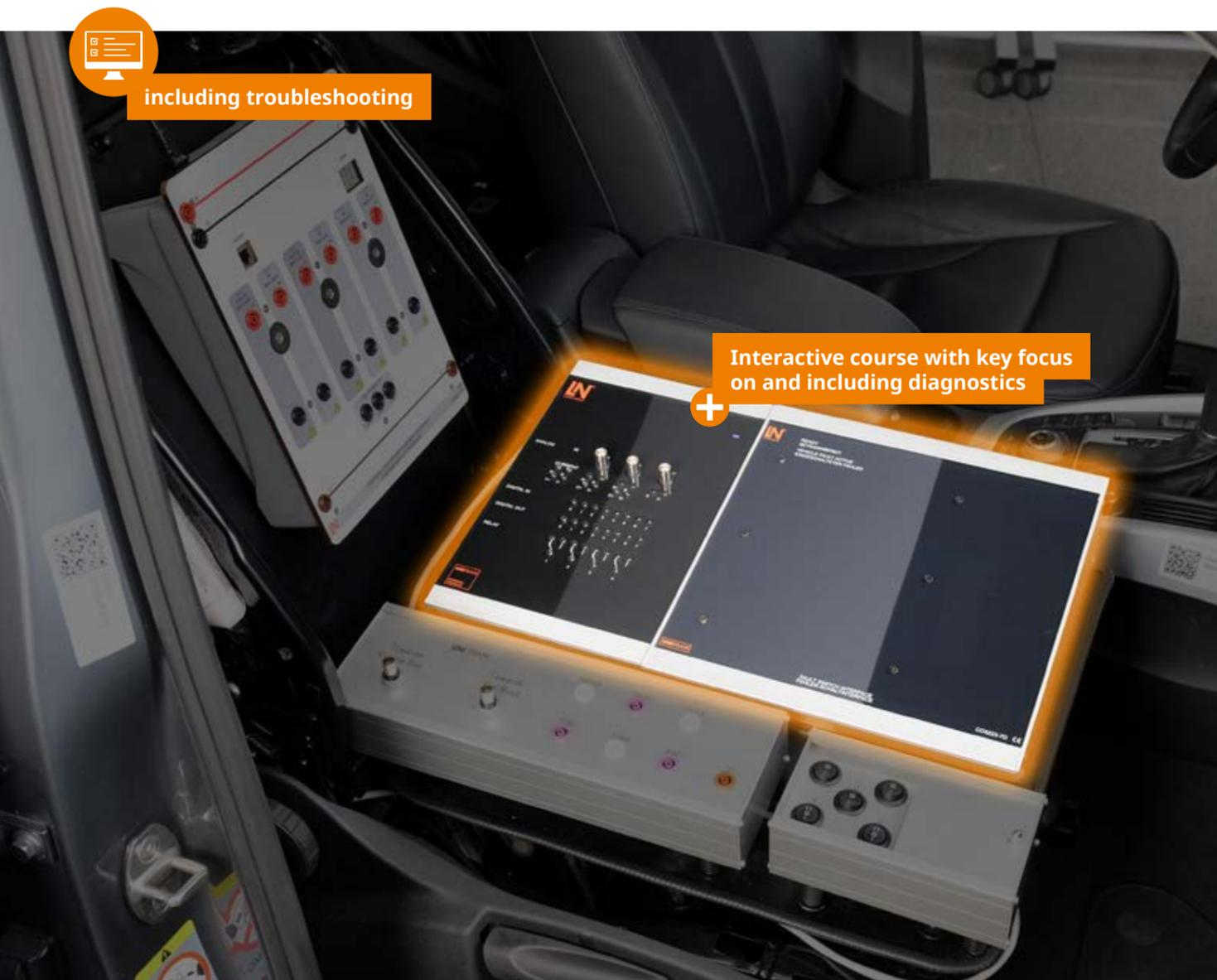
In order to bring out the full potential of our training vehicles, we recommend installing the digitisation package. This set equips a vehicle with a WiFi-capable measurement and diagnostic interface, allowing simulated faults to be activated and measurements to be saved to the learning environment. All the measuring instruments (4-channel oscilloscope, multimeters, current probe etc.) are already built in and can be comfortably started from the learning environment, thus saving space.
