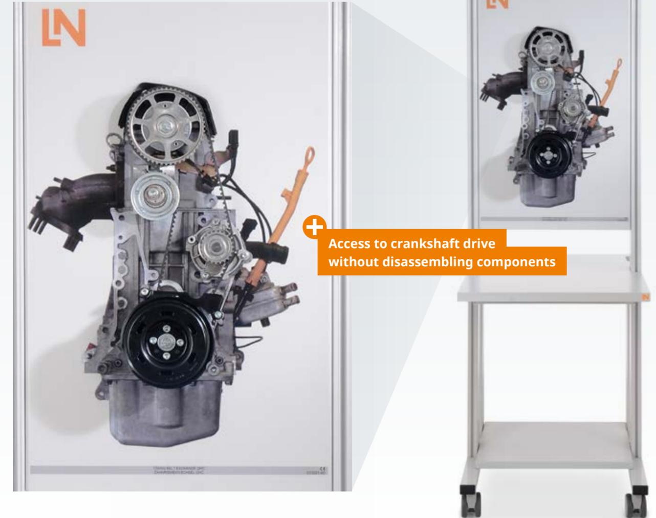
Changing toothed belts is one of the key jobs to be carried out when servicing vehicles controlled using such belts. It is particularly important to keep the timing accurate and not to change the position of the camshaft with respect to the drive shaft. This training system teaches you the best and safest way to change a timing belt.
