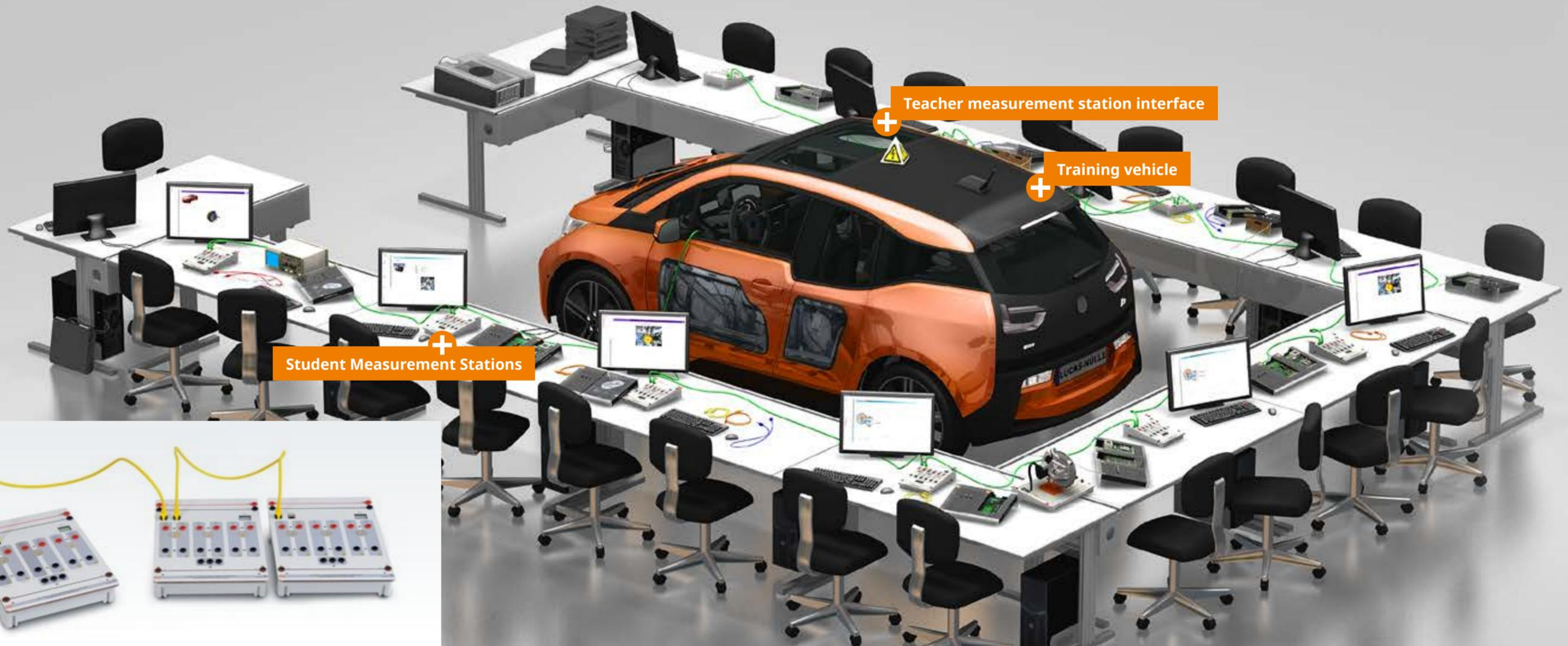
Flexibly interconnectable and secure student measuring stations. This system also provides trainees with the required signals. The source of the signals can be any electrical system, whether it be the training system itself or a real vehicle.
