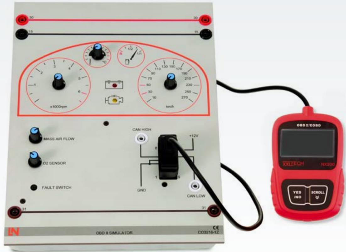
Read out data from components related to exhaust emissions with the help of on-board diagnostics (OBD II or EOBD). This system shows how OBD testers should be properly used and how to make optimum use of their functional capability. The course also focuses on correct interpretation of fault readouts.
