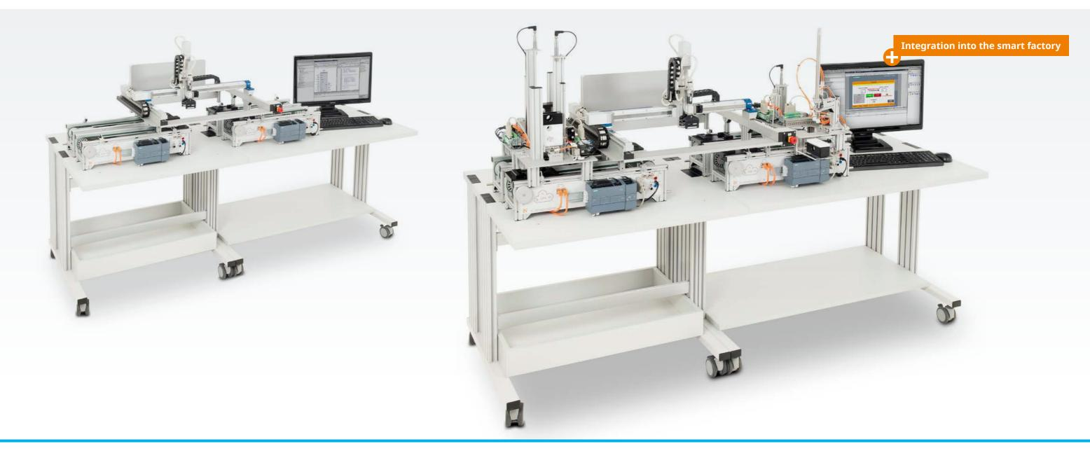
The gantry robot can be fully integrated into a production line. It is also possible to use the gantry robot to expand the smart factory system (industry 4.0). This way, the 3-axis system supports the logistical operations of a production line to convey materials between individual processing phases.
