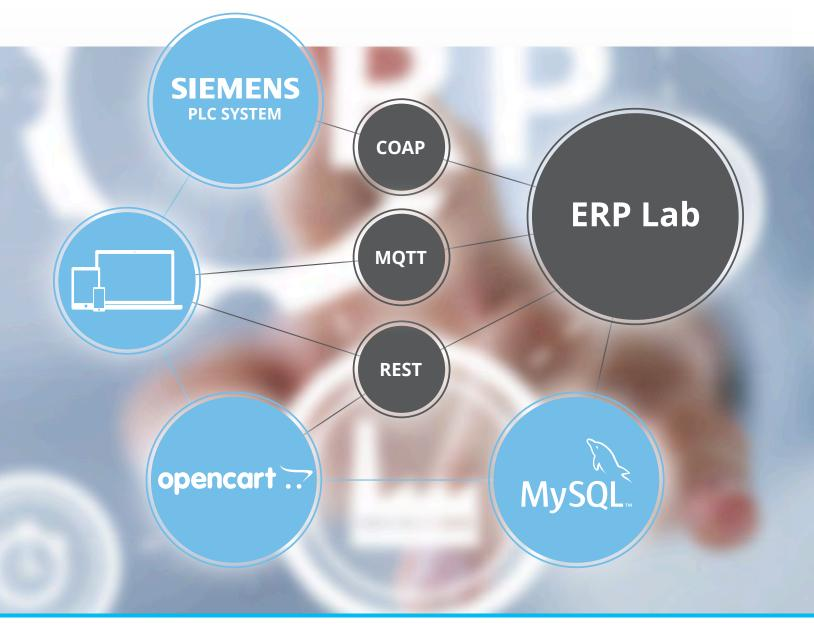
In its function as a **Manufacturing Execution System** (MES) the ERP Lab monitors the entire process. As a server-based system it provides all production-relevant data within the Edge Cloud (Cloud services in the intranet) – ranging from the Webshop to the production process all the way to warehousing. The system also communicates with the programmable logic controls of the production line via the network.
